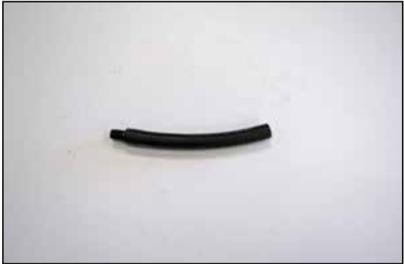
20. Install the provided union fitting into the provided crank case vent hose as shown.
