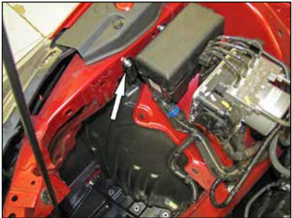
15. Remove the bolt that secures the electrical junction block to the inner fender. NOTE: This bolt will be reused in a later step.
