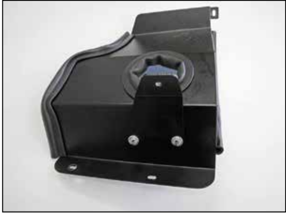
9. Install the tube mounting bracket (064336) onto the heat shield and secure with the provided hardware.
