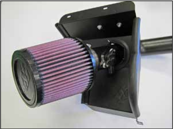
13. Install the K&N® air filter onto the intake tube and secure with the provided hose clamp.
