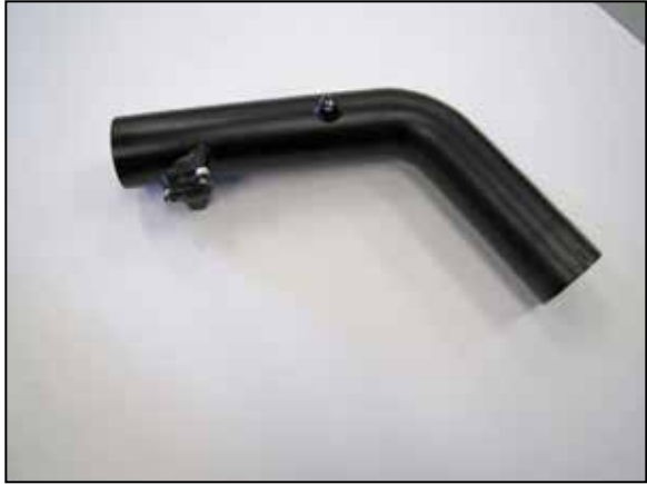
11. Install the mass air sensor into the K&N® intake tube and secure with the hardware provided.
