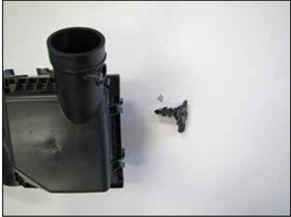
10. Remove the mass air sensor from the factory air filter housing.
