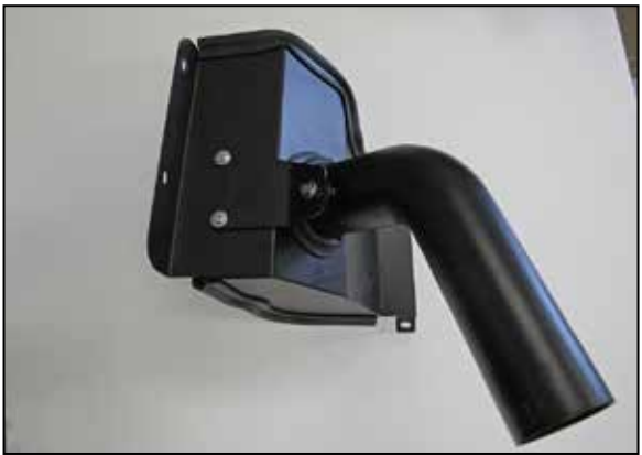
12. Install the K&N® intake tube assembly into the heat shield and secure with the provided hardware as shown but do not completely tighten at this time.
