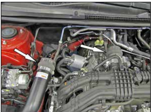
17. Install the provided hump coupler hoses onto the throttle body and the K&N® intake tube as shown and secure with the provided hose clamps.
