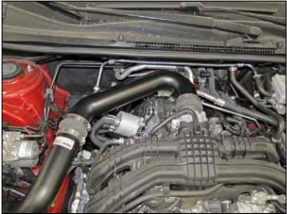
19. Install the K&N® intake tube into the hump couplers, adjust both tubes for best fit and then secure the hose clamps and the tube mount to the heat shield.
