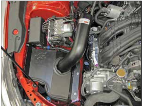
16. Plug in the mass air sensor electrical connection and then install the heat shield/tube assembly onto the rubber mounted studs and align with the electrical junction block. Secure the heat shield with the provided hardware and the factory bolt removed in step #15.
