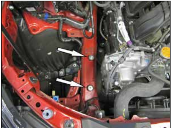
14. Install the two provided rubber mounted studs onto the frame rail where shown.
