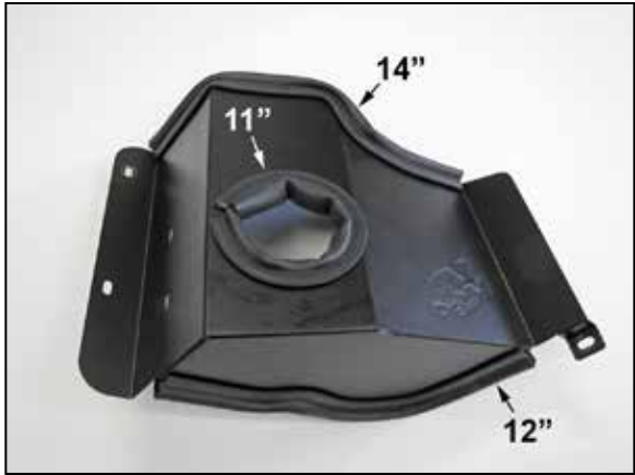
8. Install the edge trim onto the heat shield as shown.
