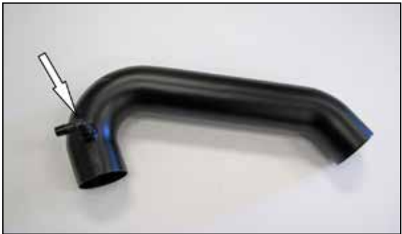
18. Install the provided 90° vent fitting into the K&N® intake tube as shown. NOTE: Plastic NPT fittings are easy to cross thread. Install the vent fitting “hand” tight, then turn it two complete turns with a wrench.
